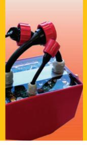
1 kWh battery module in autonomous operating vehicles for deep sea exploration
