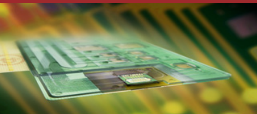
Fraunhofer ivD-cartridge equipped with electrical biochip, fluidic parts and reservoirs
