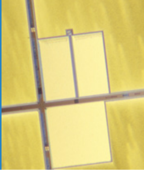
PowerMOS device with temperature sensor
