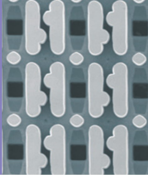
Figure 4: Deflection array realized in metal surface micromachining technology
