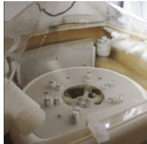
Figure 2: SSEC model 3303 single wafer etch & clean processor for metal wet etch (cleanroom view, etch chamber and disposal module)
