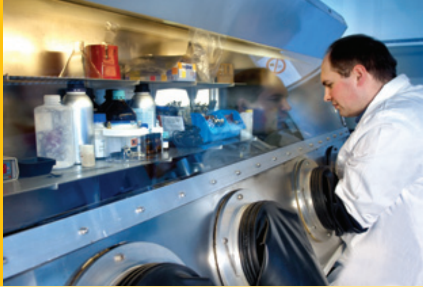
Electrolyte filling of Lithium Ion batteries in an Argon atmosphere glovebox
