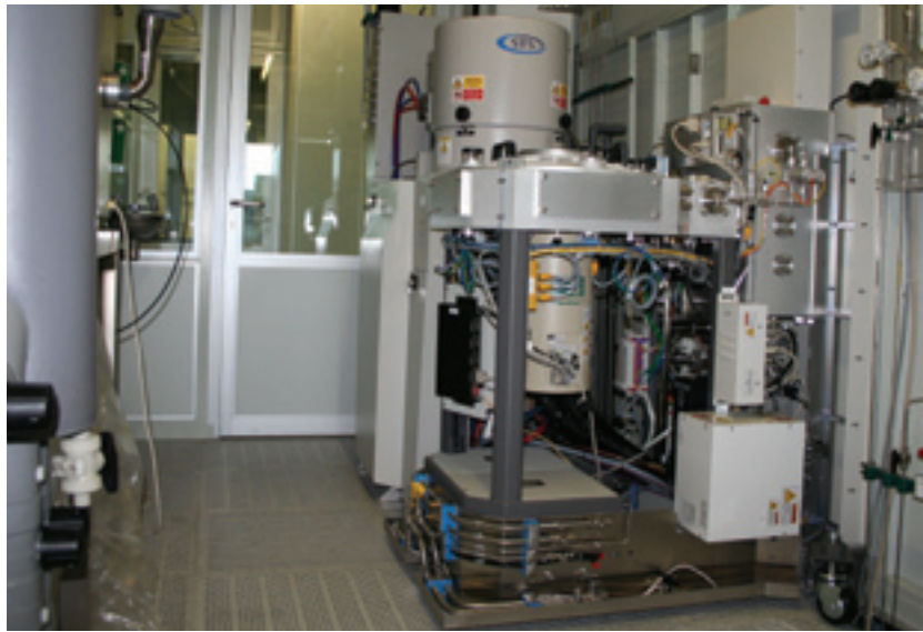
Figure 2: SSEC model 3303 single wafer etch & clean processor for metal wet etch (cleanroom view, etch chamber and disposal module)
