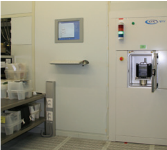
Figure 2: SSEC model 3303 single wafer etch & clean processor for metal wet etch (cleanroom view, etch chamber and disposal module)
