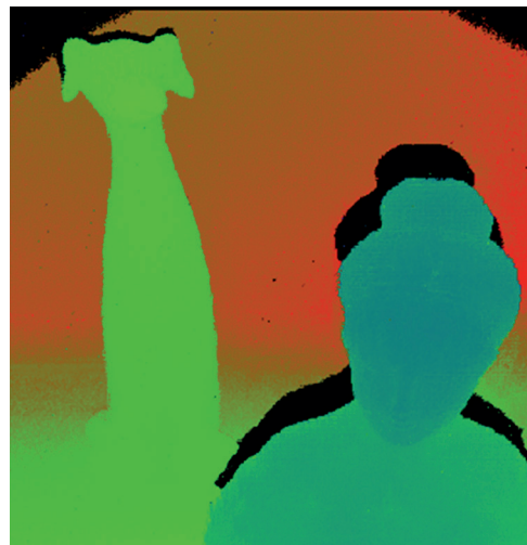
Different working modes of the camera. Left: Reflected light intensity. Right: Phase shift between light source and reflection.
