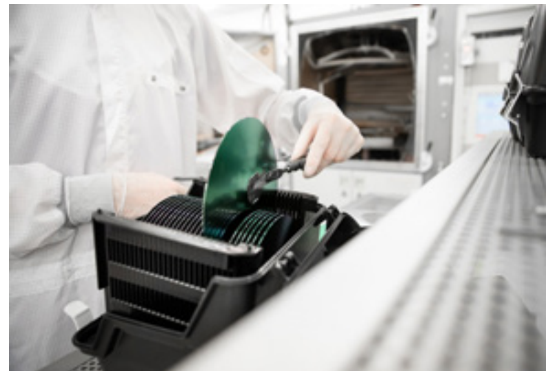
Handling of 8-inch wafer in clean room
