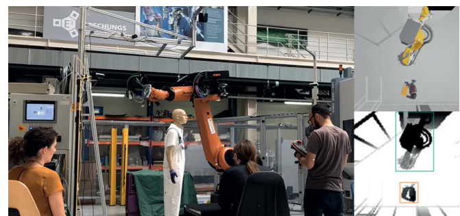
NeuroSmart scientists gathering training data on current sensor hardware (left) and 3D modeled digital twin with simulated sensor depth data as well as annotated objects (right).
