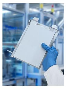
Accumulator cell with reference electrode
